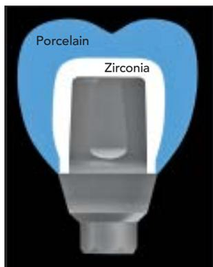
**Fig 1** Schematic drawing of standard  $ZrO_2$  screw-retained restoration, where the veneering porcelain is blocking the zirconia from contact with peri-implant tissues.
